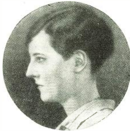
From a photograph of a subject being televised by the Ives system. The dark bands caused by the edges of the circular holes are visible.
