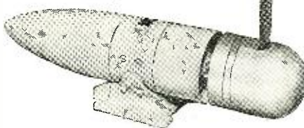
The generator of current for the airplane transmitter, showing the single vane which rotates it, by air pressure, when the plane is flying.
