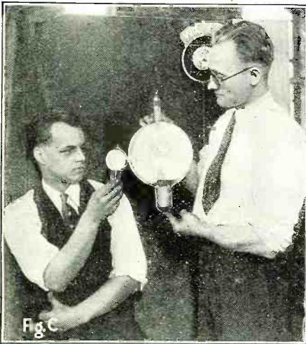
U. A. Sanabria, left, and V. A. Schoenberg, right, showing the difference in size between an ordinary photoelectric cell and the large type used at WCFL.
